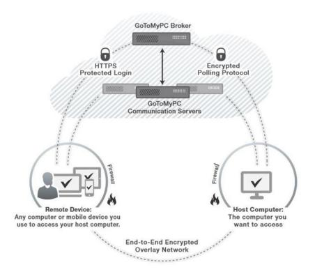
The infrastructure is designed in a manner intended to be both robust and secure. Redundant routers, switches, server clusters and backup systems are designed and employed to ensure high availability. For scalability and reliability, switches transparently distribute incoming requests among web servers. For the purposes of ensuring optimal performance, the GoToMyPC broker load balances the client/server sessions across geographically distributed communication servers.
